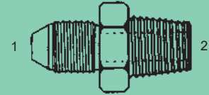
JISBP-MP-2404 - Str. (1) Male 30° BPP (Flare) (2) Male NPT Pipe
